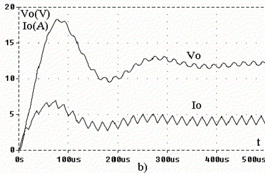
Figure 6: Simulation results of a step-up transient process for the buck converter in a closed loop system. a) Matlab-Simulink s - and z -models, b) PSPICE simulation.
