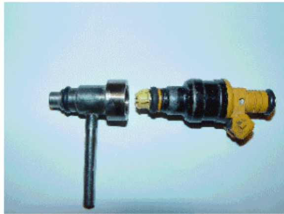
Figure 6: General view of the tested atomizer (on the left) and the serial atomizer (on the right).
